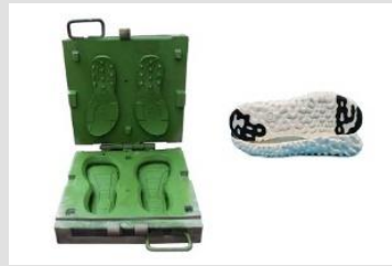
Co-molding Process of EVA & Rubber Sole
